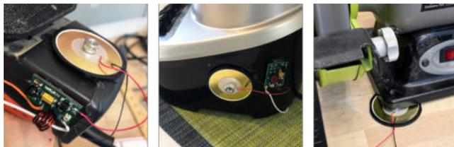
Figure 2. Sozu-augmented objects that convert energy from vibration: sander, blender, and grinding wheel.
