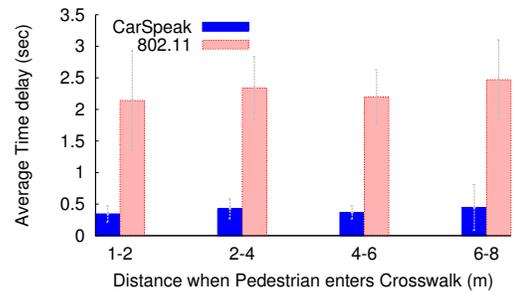
**Figure 18—Time Delay Averages for CarSpeak and 802.11.** Distances on the x-axis are grouped into bins of two meters representing distances of the golf car from the crosswalk at the time the pedestrian enters the crosswalk.
