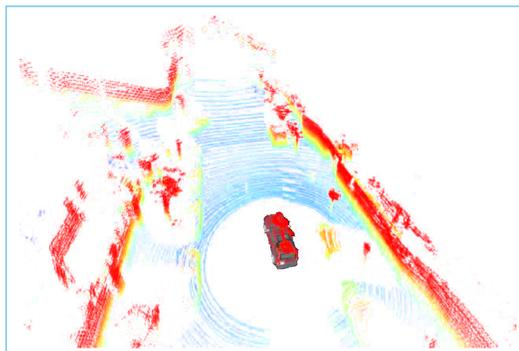
**Figure 1**—Example of sensory information used in autonomous driving. The figure shows a 3D-point cloud of a road obtained by a Velodyne laser sensor, where colors refer to elevation from the ground. Note that a 3D-point cloud provides the  $(x, y, z)$  coordinates of points lying on the surface of obstacles.
