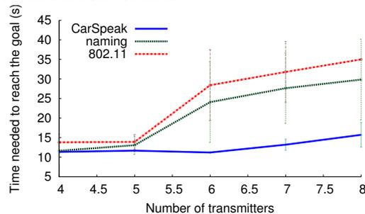
**Figure 16—Planning Efficiency.** Time taken by the robot to navigate an obstacle ridden environment across number of contending wireless nodes. CarSpeak performs 2.4× better, on average, than the baseline 802.11 implementation in a network of over 6 robots.
