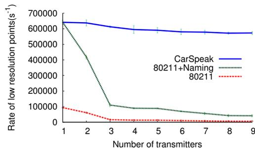
**Figure 14—Resolution.** The figure shows the rate at which information is received from a requested low-resolution region, for different schemes. Increasing the number of robots that do not have the requested resolution can dramatically impact the performance of 802.11 and 802.11+Naming. In contrast, CarSpeak maintains high rate of information from the desired region.
