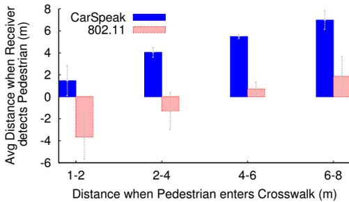
**Figure 19—Comparison of golf car distance from the crosswalk when the pedestrian enters the crosswalk to the distance from the crosswalk at which the receiver issues a stop command to the car. Distances on the x-axis are grouped into bins of 2 m.**
