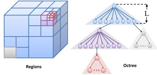
**Figure 5—Naming Regions in CarSpeak.** The figure on the left shows four different regions at different hierarchies with  $L = 2$ . The figure on the right depicts the truncated sub-trees corresponding to these regions in the Octree.
