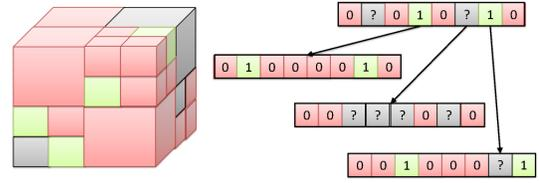
**Figure 6—Octree Representation** Representation of 3D-point cloud using a 2-level Octree. Vertices that are unoccupied are not expanded; vertices that are completely occupied or unknown are terminated by special leaf vertices; these have been omitted for clarity.
