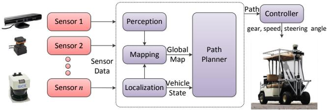
**Figure 3—High-Level Architecture of Autonomous Vehicular Systems.** The path planner module uses information from various sensors to compute a safe path for the vehicle.
