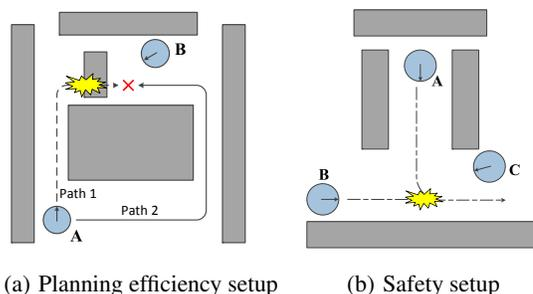
**Figure 15—Experiment setup** for (a), The shortest path 1 from A to destination is blocked, efficient communication from sensor B should enable A to take path 2; for (b), There is a potential collision of A with B when A tries to merge into the traffic in another road at the T intersection. The collision can be avoided if A can hear from C about the other side of the road.
