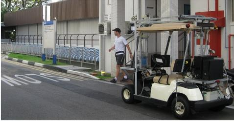
**Figure 9—CarSpeak’s Outdoor Setup.** Image of the actual golf car route demonstrating the lobby area that poses a hazardous blind spot for the golf car and makes visual confirmation of a pedestrian difficult before he enters the road.
