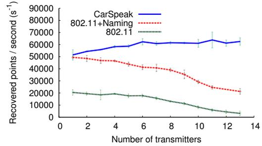
**Figure 12—Scaling.** Number of 3D points received at a receiver by CarSpeak, 802.11 and 802.11+Naming as a function of the number of contending nodes. We observe that while CarSpeak scales gracefully, 802.11’s performance deteriorates when there are over 6 nodes, due to an excessive number of collisions and the lack of a backoff mechanism in the broadcast mode.
