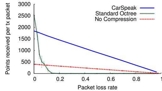
**Figure 13—Compression module.** Ratio of the number of points received over the number of transmitted points measured across packet loss rates when packetizing compressed point cloud data, using CarSpeak’s compression module and without using compression. CarSpeak’s compression module provides a consistent gain of 4.5x over sending uncompressed data, while packetizing compressed point cloud data performs poorer than CarSpeak for packet loss rates as low as 2%.
