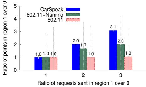
**Figure 11—Region Requests.** Ratio of the number of points received from two requested regions plotted against ratio of the number of requests made for the two regions. CarSpeak ensures the wireless bandwidth is allocated to region proportionally to the number of requests they receive.
