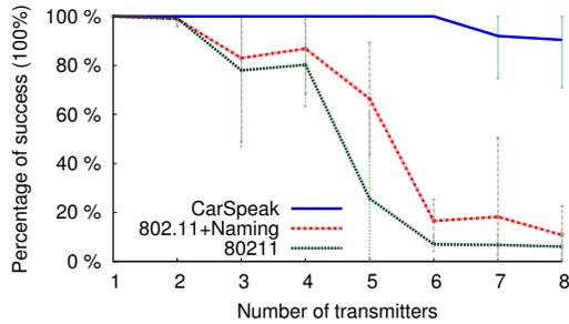
**Figure 17—Safety.** Percentage of successful detection of Robot B across number of wireless nodes contending for the medium. For a network of over 6 contending transmitters, CarSpeak’s probability of successfully detecting Robot B is  $14\times$  that of 802.11 and  $6.5\times$  that of 802.11+Naming.
