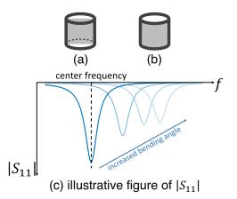
Figure 5: Instead of design (a), NFCapsule adopts design (b) to wrap a bent coil around the capsule to obtain a larger coil area, although this may sacrifice some coil performance (c).
