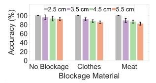
Figure 13: NFCapsule's classification accuracy on gel models with blockage. The result is grouped by material on the Xaxis; each group contains four accuracy values of different reading ranges. We see clothes and meat induce similar performance drop to NFCapsule.
