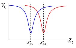
Figure 7: Illustrative curves showing the qualitative relationship between  $V_0$  and  $Z_t$  with two coils tuned to different optimal impedance values.
