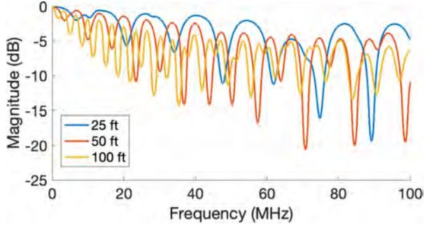
Figure 3: Reflection characteristics (S11) of cables with different lengths demonstrate the standing wave effect and attenuation trend as frequency and cable length vary.
