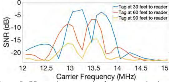
Figure 5: PLatter leverages the frequency-selective behavior of the power lines to improve the tag SNR by intelligently shifting the frequency of the carrier signal.
