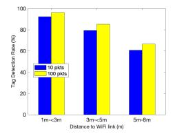
Fig. 18. Tag detection rate for different TX-RX locations.
