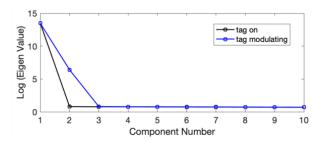
Fig. 4. Tag modulation increases the signal subspace eigenvalues which indicates the rank increase of the signal covariance matrix.
