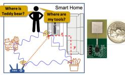
Fig. 1. TagFi's deployability and Single-point localization capabilities provides users with a WiFi-based object finding in any arbitrary environment without requiring a localization infrastructure in place.
